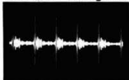
Fig. 1 SSB signal before processing. See the high peaks and the low valleys. Our NCX-3 is putting out only 25 watts average power.
