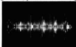
Fig. 2 SSB signal after processing with LSP-520BX. The once weak valleys are now strong peaks. Our NCX-3 now puts out 100 watts of average power.
